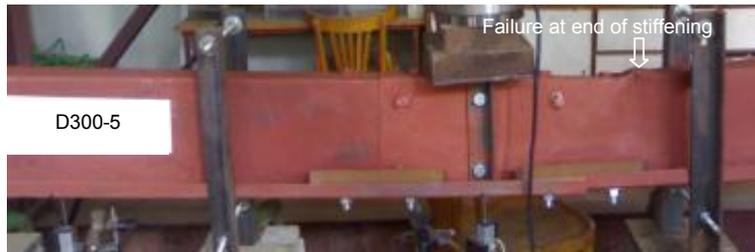
**Fig. 10. Mode of failure of specimen (D300-5)**
