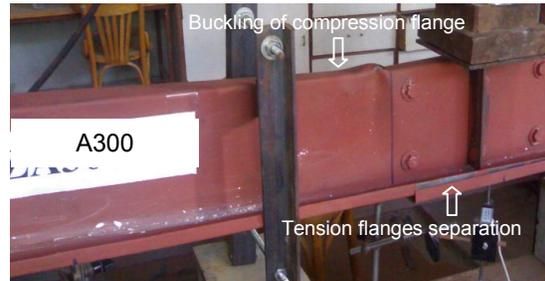
**Fig. 7. Typical modes of failure of tested specimens with bolted connections**
