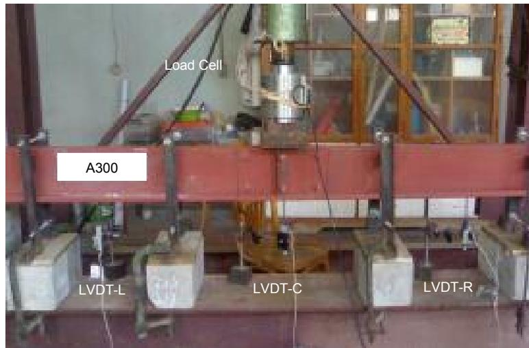
**Fig. 6. Setup of the experimental test**
