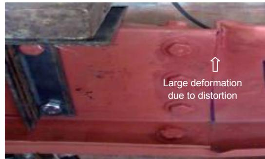
**Fig. 8. Mode of failure of specimens' series (B)**
