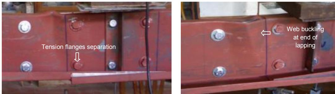
**Fig. 11. Mode of failure of specimens (D240-3 and D240-4)**
