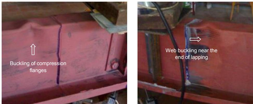
**Fig. 12. Mode of failure of specimens' series (C)**
